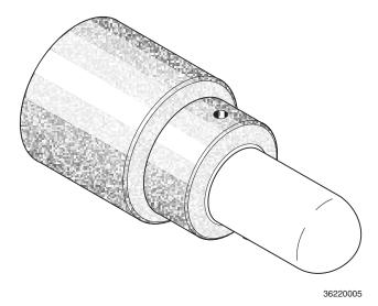
Figure 1-3. Flame Arrestor Diffusion Assembly
